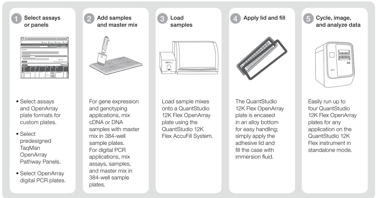
**Figure 1. SNP genotyping workflow with OpenArray plates and the QuantStudio 12K Flex System.** This workflow offers the convenience of high-throughput flexibility in conjunction with Custom TaqMan SNP Genotyping Assays. With each through-hole of the OpenArray plate having a capacity of 33 nL, reagent costs are minimized while maximizing throughput and retaining quality results.
