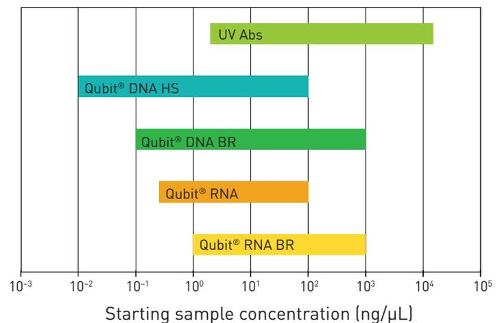
**Figure 4. Comparison of sample concentration ranges for the Qubit® assays and UV absorbance measurements using a microvolume UV spectrophotometer.**
