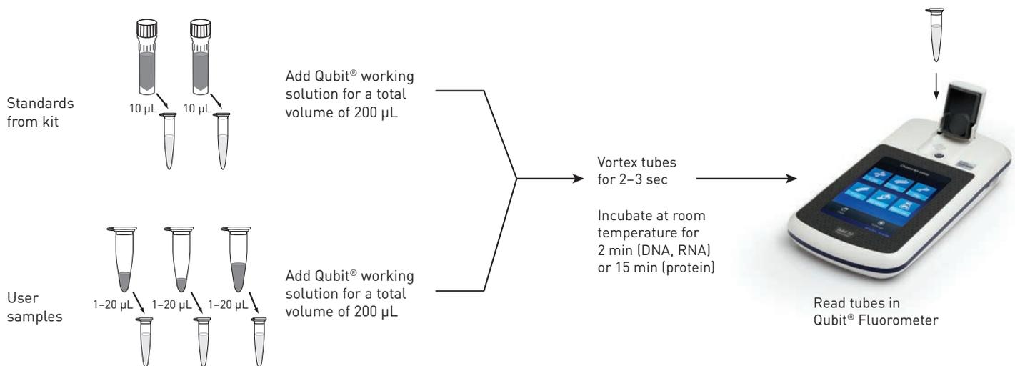
Figure 1. Workflow for the Qubit® assays using the Qubit® 2.0 Fluorometer.
