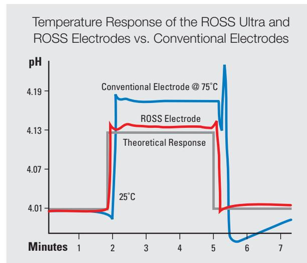
**The graph shows how ROSS electrodes respond versus the best of conventional pH electrodes.** The ROSS electrode continues to show fast reproducibility and accuracy after many dramatic temperature changes.
