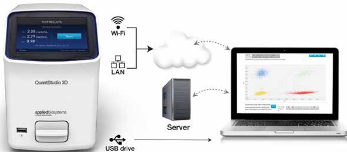
Figure 4. Primary analysis performed directly on the QuantStudio 3D Digital PCR Instrument in less than 1 minute. The instrument displays absolute quantification in copies/µL and a quality flag. Data files can be automatically transferred to QuantStudio 3D AnalysisSuite Software through a personalized, cloud-based user account on the Web. A stand-alone server can be used in lieu of accessing the cloud. An example of data analysis using the Relative Quantification Module in QuantStudio 3D AnalysisSuite Software is shown on the laptop screen. Ideal for applications such as rare allele detection, data from multiple chips can be combined to automatically display a scatter plot based on the color of rare and wild type events. For further quality control, boundaries of rare vs. wild type vs. undetermined events can be manually defined.
