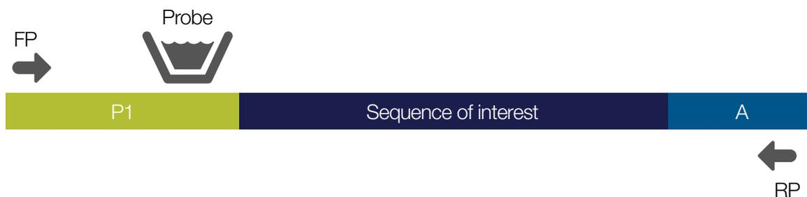
**Figure 2. TaqMan Assay design for Ion Torrent library quantification on the QuantStudio 3D Digital PCR System.** The assay is composed of a forward primer (FP), reverse primer (RP), and TaqMan™ probe all complementary to the library P1 and A adapter sequences.
