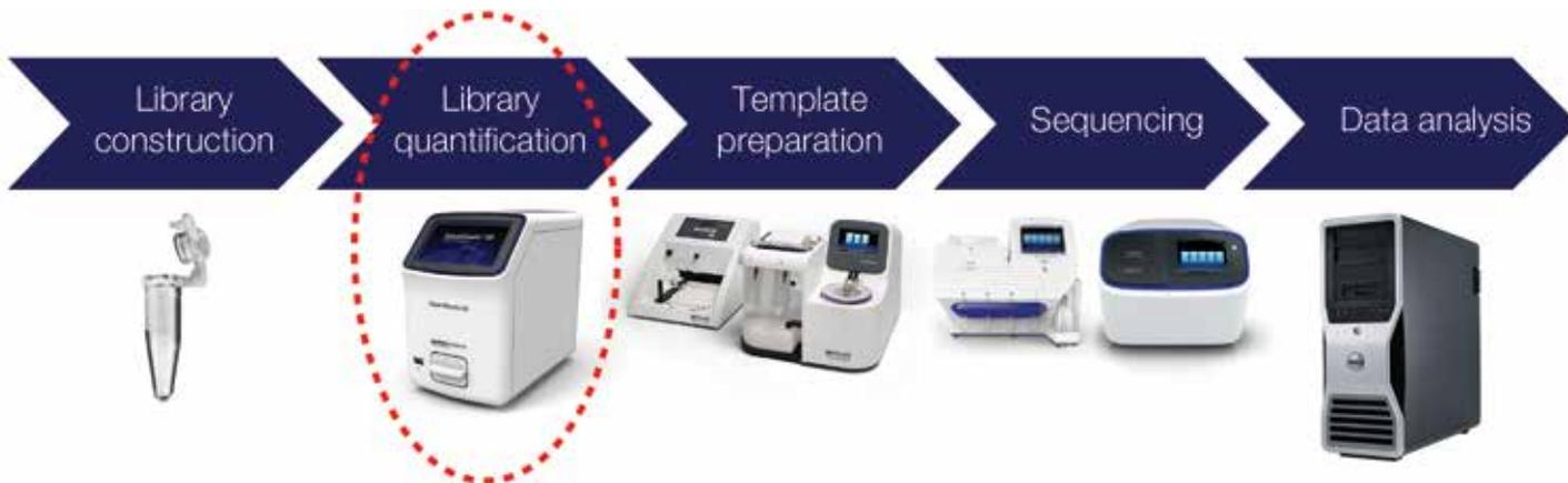
**Figure 1. NGS workflow incorporating the QuantStudio Digital PCR 3D system to accurately quantify NGS libraries prior to template preparation on the Ion OneTouch™ 2 System.**
