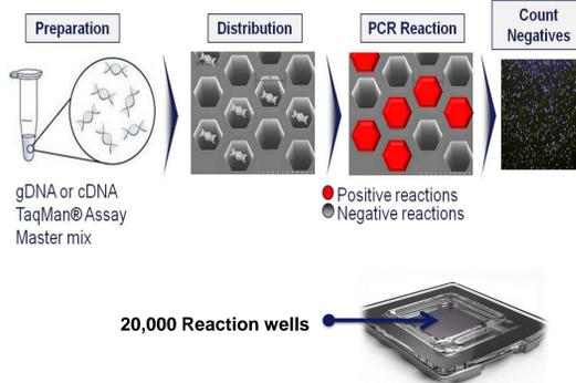
QuantStudio™ 3D Digital PCR System is based on a silicon chip that is partitioned into 20000 individual reaction wells, used for nucleic acid detection and absolute quantification. Each sample is distributed into 20,000 individual endpoint PCR reactions per chip where some of these reactions contain target molecule (positive) while others do not (negative). The fraction of negative reaction wells is used to calculate an estimation number of target molecules present.
