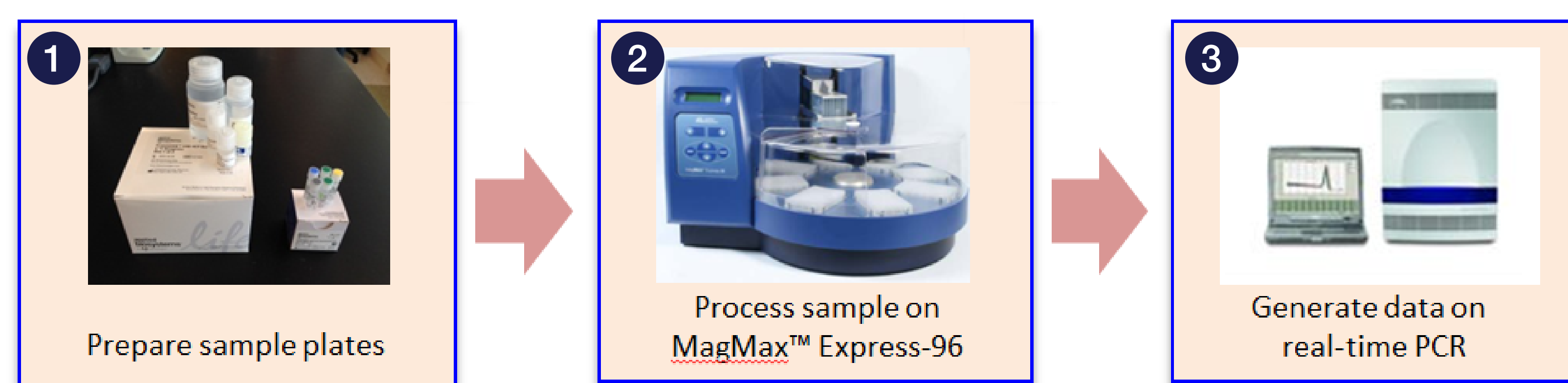
Figure 1. ProteinSEQ work flow comprises sample prep, automated sample process on MagMax instrument and qPCR data acquisition.
