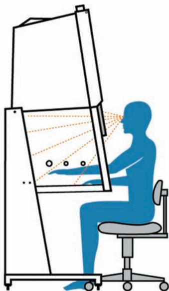
**Figure 1.** Choosing a biological safety cabinet with many ergonomic design features can improve operator comfort. An angled front promotes a more natural head and elbow working position, which allows the operator to get closer to their work, extend their reach and assume a comfortable and relaxed working environment.
