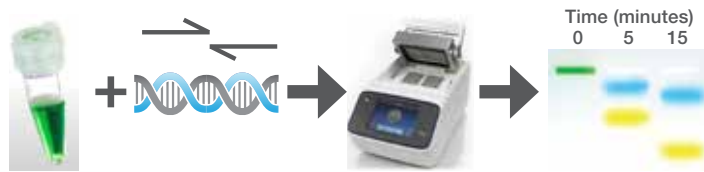
Figure 2. Simplified PCR workflow. Convenient Invitrogen™ Platinum™ Hot Start Master Mixes reduce the number of steps during PCR reaction setup. Green buffer enables direct gel loading of PCR products, eliminating tedious steps of dye addition. Left lane of gel image shows reaction mixture with green buffer prior to electrophoresis. Right lanes of gel show yellow and blue dye migration following 5 and 15 minutes of electrophoresis.
