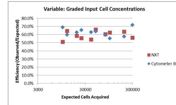
In this data set, cell density does not have a major effect on acquisition efficiency. Both the Attune NxT and Cytometer B had an average efficiency of around 60%. Higher cell densities did result in greater variability in efficiency as reflected in larger standard deviations. Technical difficulties prohibited including Cytometer C in this data set.
