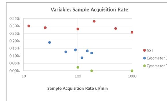
Sample carryover after 2 washes was independent of sample acquisition rate and acceptable on all instruments (<0.35%), but was lowest on Cytometer C, which has the simplest and most direct fluidic system.
