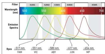
Figure 1. Fluorescence emission spectra of different dyes used for multiplex PCR.
