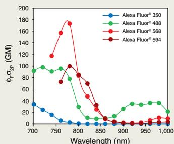
**Figure 3—Two-photon excitation spectra of Alexa Fluor<sup>®</sup> 350, Alexa Fluor<sup>®</sup> 488, Alexa Fluor<sup>®</sup> 568, and Alexa Fluor<sup>®</sup> 594 dyes.** The y-axis units are products of fluorescence quantum yields ( $\Phi_f$ ) and two-photon absorption cross-sections ( $\sigma$ ). Data courtesy of Warren Zipfel, Cornell University.
