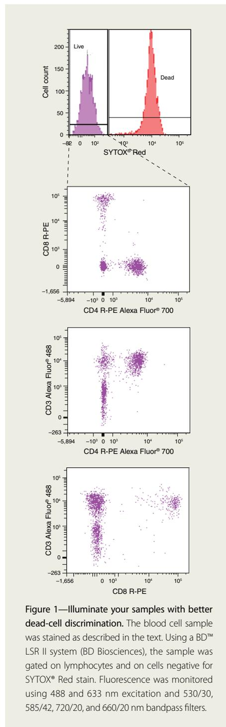
**Figure 1—Illuminate your samples with better dead-cell discrimination.** The blood cell sample was stained as described in the text. Using a BD™ LSR II system (BD Biosciences), the sample was gated on lymphocytes and on cells negative for SYTOX® Red stain. Fluorescence was monitored using 488 and 633 nm excitation and 530/30, 585/42, 720/20, and 660/20 nm bandpass filters.
