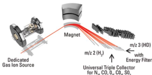
▲ A range of components—including a magnet, filters, and collectors—make isotope ratio mass spectrometry work. (Image courtesy of Thermo Fisher Scientific.)
