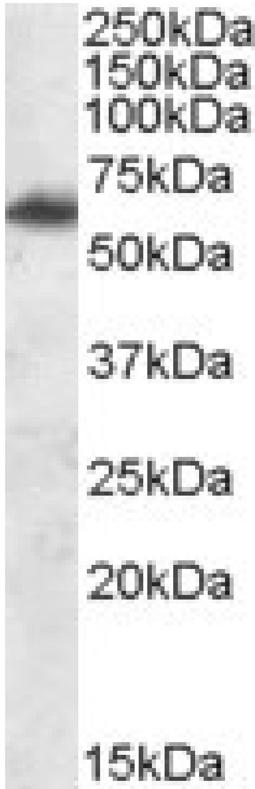
FTO Antibody (PA5-18942) in WB Western blot analysis of FTO using FTO Polyclonal Antibody (Product # PA5-18942) (0.03 µg/mL) in staining of Human Pancreas lysate (35 µg protein in RIPA buffer). Primary incubation was 1 hour. Detected by chemiluminescence.
